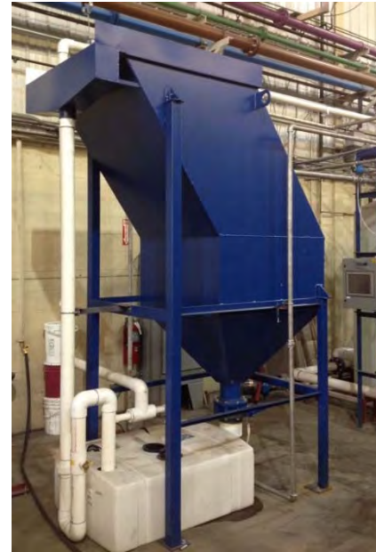
Lamella Clarifier Scale Model
